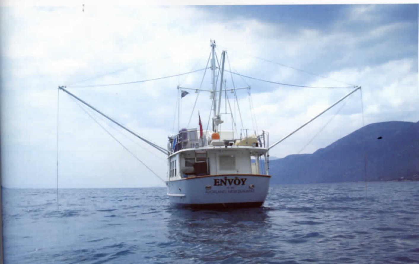
ENVOY'S STERN SHOWING THE PARAVANES DEPLOYED. A STEEL PLATE, OR "BIRD", IS TOWED ABOUT 5M UNDER WATER EACH SIDE TO REDUCE ROLL. THE VARIOUS LINES KEEP THE PARAVANES IN PLACE.
