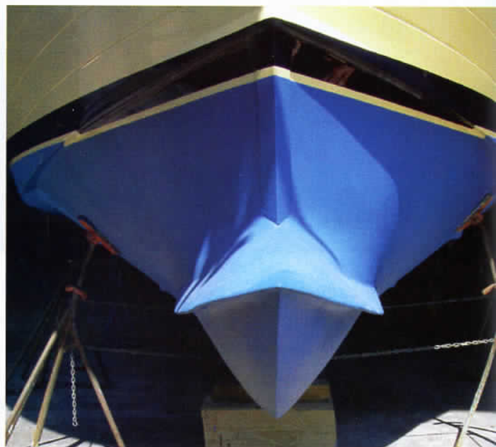
Marlow's Rebel Yell features a hybrid wave piercer bulb that helps calm vertical acceleration while it begins deflecting oncoming water.
