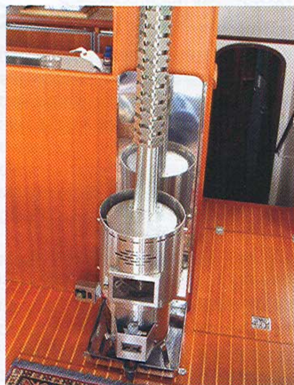
A gravity-fed diesel heater will help keep the chill off on those cold nights
